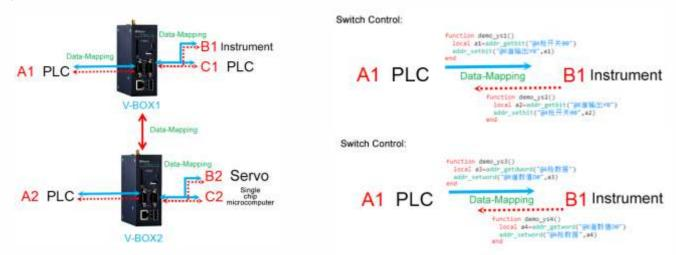
**Network mapping**: Realize mutual control and data interaction of multiple COM ports between multiple V-BOX by this mode; Synchronous monitoring and operation.
