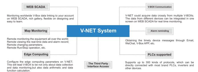
WECON OPC Tool and HTTP API, could help the third party server to acquire data from V-NET, such as MES, ERP, the After-Sales System, the Tractability System, etc.
